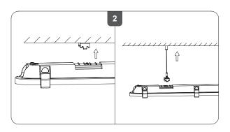
2. Position and fix base using the pre-fixed mounting brackets / suspension kits.
