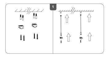
1. Identify installation location & check for any passing wiring/piping prior drilling and installing cables. Fix the mounting brackets / suspension kits on the ceiling at correct spacing as per dimensions.(Pic.A)
