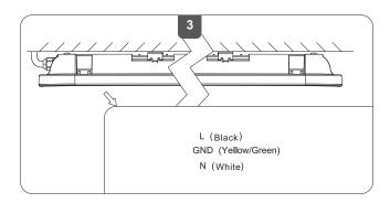
3. Connect the power cable accordingly.
